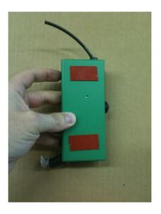
Carefully line up the transmitter with the lower right hand side of the remote box. Make sure that everything is lined up before applying any pressure to the transmitter as it will cause the double-sided tape to cure.
