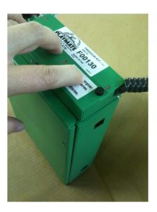
4. Plug the short retractable cable into the remote box. No other cables are needed.
