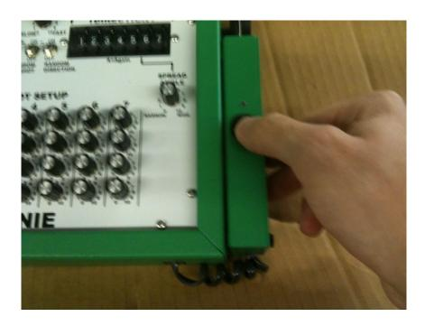
Any time you change any settings on the remote box, you need to press the black button on the FREEDOM KIT Transmitter to send the updated settings to the ball machine.
