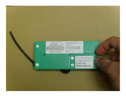
2. Replace the batteries with 2 AA Energizer "LITHIUM" type batteries. Do NOT use alkaline batteries. If you can't find Energizer batteries, make sure that the batteries are of LITHIUM type.
